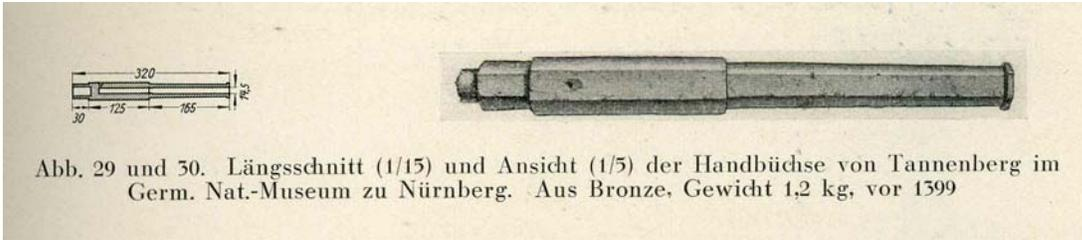
Figure 15. Drawing and dimensions of early handgun from the Tannenberg Castle in Germany. This handgun, which weighed 1.2 kilograms, was manufactured out of bronze at some point before 1399; the dimensions are in millimeters. Source: Rathgen, illustrations 29 and 30.
